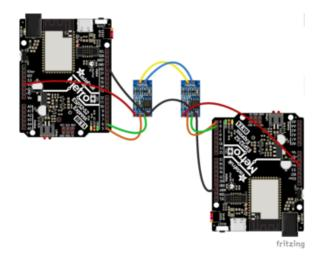
Metro V<sub>HI</sub> to Transceiver VCC Metro IO5 to Transceiver TX Metro IO6 to Transceiver RX Metro GND to Transceiver GND Make the following connections between the two transceivers:
