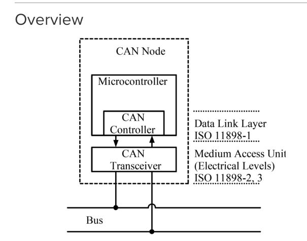
In this guide you'll learn how to use CircuitPython's **canio** module to send and receive data between two supported boards, such as the Feather M4 CAN.
