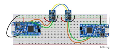
After reviewing the CAN breakout board I used, I made the following connections between each Feather and its Transceiver:
