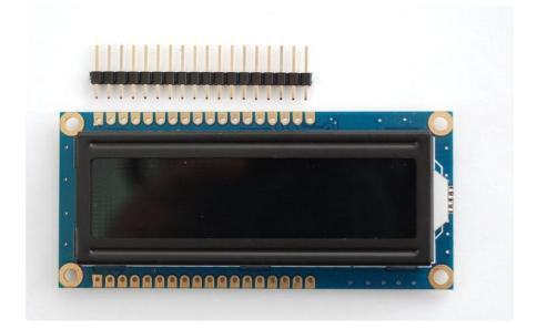
Place the header with the long side down into a breadboard. then place the LCD on top. If you're using an LCD with two rows available, make sure you're using the row that matches the image below.
