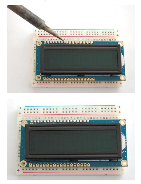
Next, align the backpack so that it matches up with the corner of the LCD, the hole in the backpack should be in the same location.
