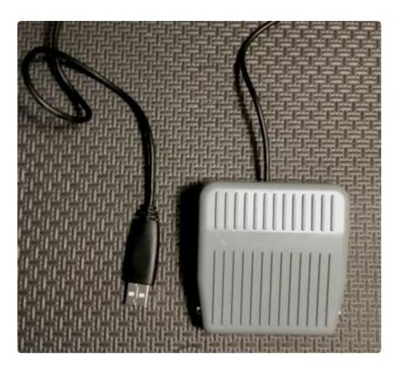
The USB foot switch should work with Windows, Linux, or Mac from the last few years (with plug and play, which has been around for quite a time). When you plug in the USB cord, the computer will detect something is plugged in but it will not know it's the switch until the Trinket boot code finishes timing out in a few seconds. Then your operating system device list will show a keyboard device entitled "Trinket Keyboard".
