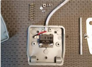
Note the cable restraint - black with 2 screws, holding the cable onto the pedal base in the above picture. Using your screwdriver, carefully remove the two screws and the black plastic bracket holding the wire. Do not remove the switch assembly in the center of the base yet.
