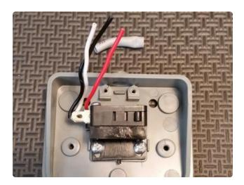
You can carefully grab the grey outer plastic of the short cut cable and slide it off revealing three wires: black, white, and red.
