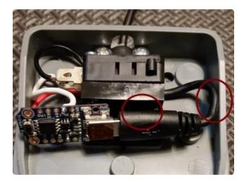
Tuck the Trinket and the cable up next to the switch. The top of the trinket board should not protrude above the switch so it will need to be placed at a slight angle. Put some pressure on the cable so the edge of the Trinket does not overlap the side of the pedal base.
