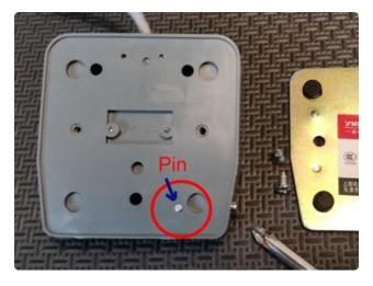
Turn the pedal over and using a medium Phillips screwdriver, carefully remove the metal back cover.
