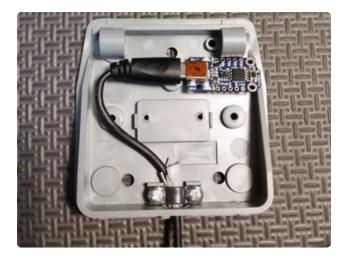
Feed the Mini-B side of the cable through the enlarged hole. Place the Trinket 5V onto the cable end to get a feel for how much cable you want inside the housing (it is a tight fit).
