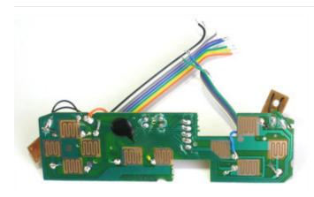
If you haven't yet, now is a good time to desolder the SNES connector cable. We wont have space for it so just pull each wire as you heat the solder joint (or just cut them short, either way).
