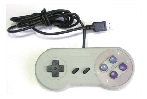
We'll start by turning the buttons of the game pad into keyboard buttons, so that pressing 'up' is converted into the 'U' key, for example. The firmware is easily adaptable, so you can adjust it for whatever software it will be used with.
