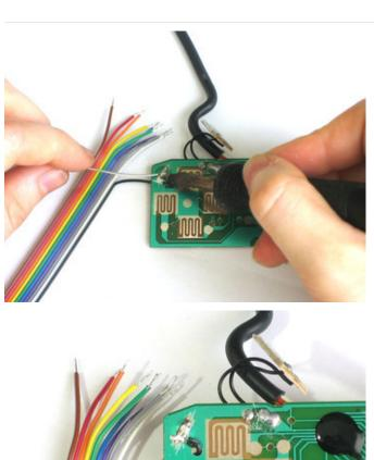
Solder the Black wire to the ground plane, we brought the wire through a hole.
