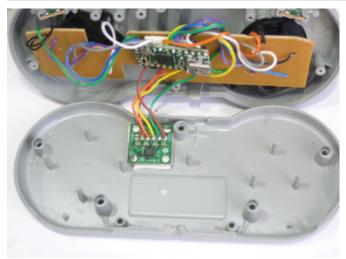
Likewise, align the acellerometer so that it is as shown (otherwise you may have some flipped axes. You should put it near the middle but we didn't see any difference being in this location.
