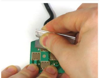
To connect to ground, we'll expose a little copper in the top left corner, this way we don't have the wire running underneath the elastomer.
