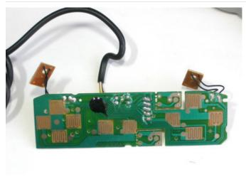
Each button is made of 3 parts - theres the plastic part that you press, beneath that is the *elastomer* which is a rubber molded piece with a conductive bit that goes underneath the plastic part, and finally on the PCB there are two interdigitated and exposed traces. When the user presses the plastic button, it pushes down on the elastomer which then pushes the conductive rubber onto both traces, shorting them.
