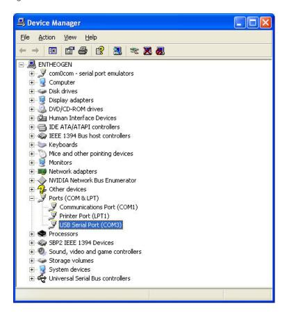
The Arduino is a USB serial port - it appears under Ports here, not under Keyboards!
