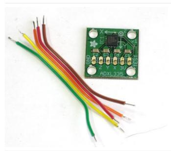
Cut a piece of ribbon cable down, we'll use Brown for Ground, Red for +3V, then Orange Yellow and Green for X Y and Z respectively.
