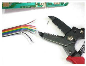
Cut off a strip of ribbon cable, about 4" long. Use diagonal cutters or fingernails to carefully nip and 'rip' the individual wires apart about 1" and then strip the ends and tin them with solder. Do this for both sides.
