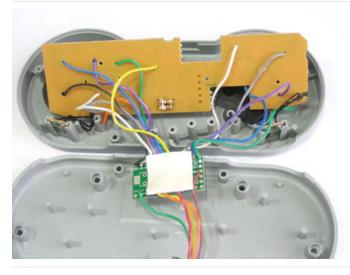
Use sticky foam tape or hot glue to place the Teensy right at the top.
