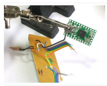
OK! Now all the buttons are wired up, its time to attach them to the Teensy. Place the Teensy in a vise or carefully use a 'third hand' to hold it (grab by the USB connector).
