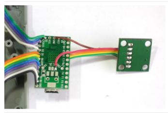
The ADXL335 requires 3V power, so don't connect it to VCC (5V) instead, we'll use the 3V that the teensy provides - it uses that voltage for the USB communication, you can't draw more than maybe 20-40mA which is plenty for this but not enough for perhaps a bunch of LEDs! Brown connects to the second GND pin.
