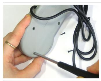
There are 5 small phillips screws on the back. Once you lift the back off, you can remove the PCB. Be careful as there are tiny wires for the 'side' buttons so just make sure those pieces come out cleanly.
