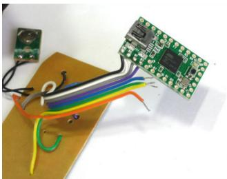
Next start soldering in all the ribbon cable wires, one after the other, without skipping any holes.
