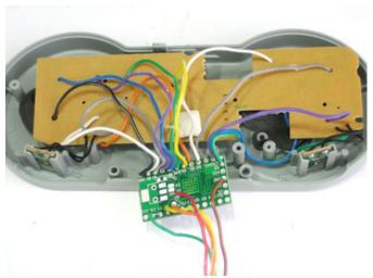
One thing that will help is 'deribboning' the ribbon cable, so that it is easy to push around the wires.
