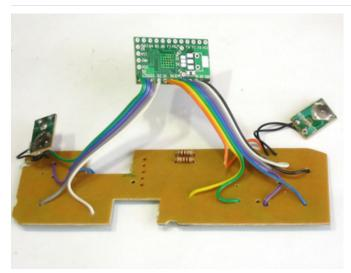
After the first ribbon cable, go to the second piece, starting with the white wire. The last green wire goes next to the blue one on the 'short' side.
