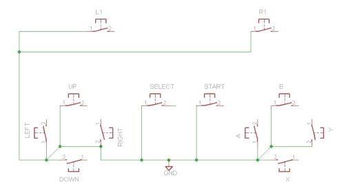
Note that this is really just a symbolic schematic, the ground wire doesn't necessarily connect on the side thats indicated, we're just showing how all the buttons have a common ground pin!
