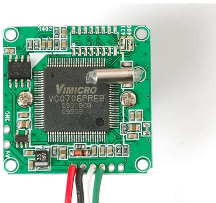
If you'd like to get NTSC video out to connect to a TV or monitor, solder another black wire to the second Ground pin, and a yellow wire to the CVBS pin.
