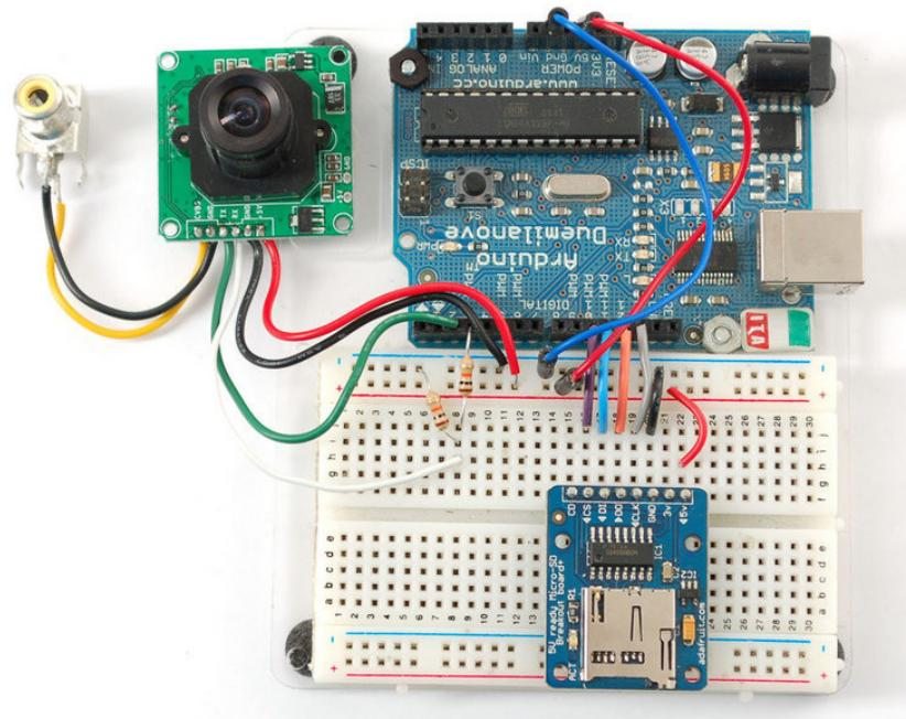
For the weatherproof camera, the white and green wires are swapped on some cameras! So please flip the white and green wires indicated if using the metal camera. Red should still be connected to +5 and Black to Ground
