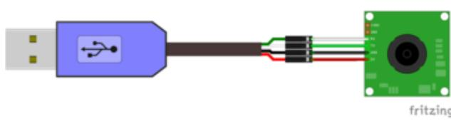
**Camera Vin to USB 5V or 3V** (red wire on USB console cable)
