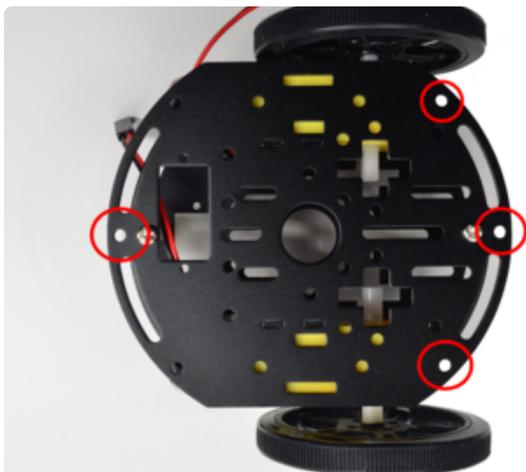
Screw the remaining 2 or 4 standoffs into the second chassis layer.
