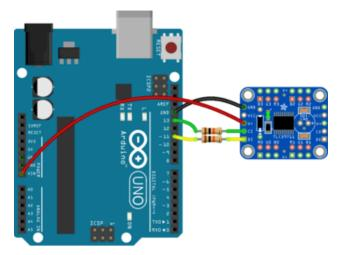
Connect V+ to 4-17V and keep VCC disconnected. Then use 10K resistors or a level shifter between the clock and data wires going into the first of the TLC59711
