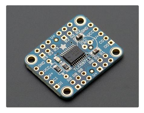
The TLC5947 has even more channels. It can control 24 separate channels with 12-bit PWM output.
