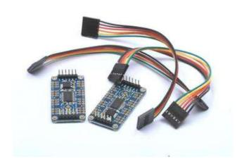
Header connections at both ends of the board make chaining simple. Our 6-Conductor 0.1" Socket-Socket Cable (http://adafru.it/206) is perfect for linking them together.
