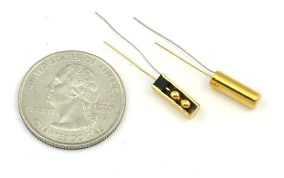
Tilt switches used to be made exclusively of mercury, but are rarer now since they are recognized as being extremely toxic. The benefits of mercury is that the blob is dense enough that it doesn't bounce and so the switch isn't susceptible to vibrations. On the other hand, ball-type sensors are easy to make, wont shatter, and pose no risk of pollution.
