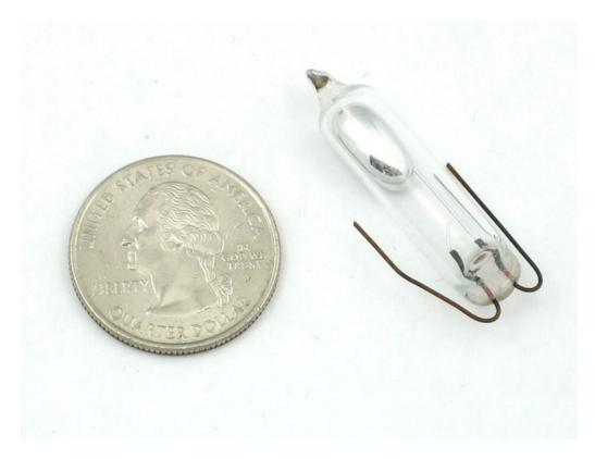
While not as precise or flexible as a full accelerometer, tilt switches can detect motion or orientation simply. Another benefit to them is that the big ones can switch power on their own. Accelerometers, on the other hand, output digital or analog voltage that must then be analyzed with extra circuitry.
