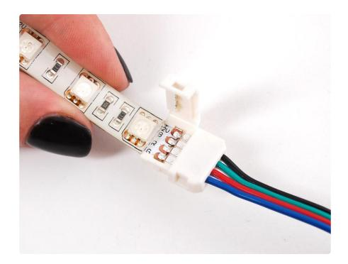
Open the plastic cover on the clip and slide the freshly sliced end of RGB LED strip under the metal tabs inside the connector.
