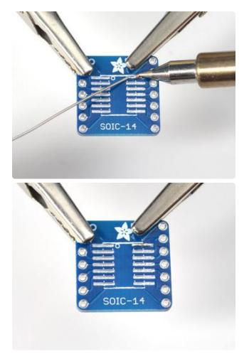
We'll start by melting a little solder on one corner pad. I like going with the top right corner. Melt just a tiny bit on, so its rounded but not blobby
