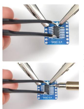
Once you've identified which is pin 1, hold the chip with the tweezers over the pads and then re-heat the corner pad you soldered onto a few steps ago.
