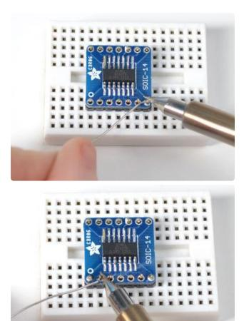
Almost done, now all you have to do is solder each header pin into the corresponding hole to make a secure connection
