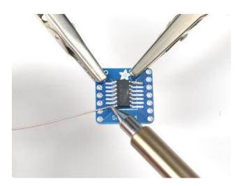
Now you can 'fix' the chip in place by soldering in the opposite corner. The one pin you soldered will keep the chip in place mostly, so you just have to solder the other pin a little to make the setup secure
