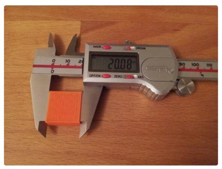
Scale calibration illustrates the process in which you compare the desired dimensions with the actual dimensions your printer produces. The easiest method for accomplishing this is to start by printing a calibration object, like a <u>Calibration</u> <u>Cube</u> (https://adafru.it/cos) or the <u>Calibration Vector</u> (https://adafru.it/cot). Once complete, use a set of calibratio to check the dimensions and record your results.
