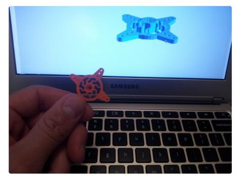
In order to produce 3D printer compatible objects, it is important to understand its limits. I like to think of a 3D printer as a spaghetti machine. It carefully stacks noodles on top of each other, and if there isn't enough noodle to stack on, it droops. The
