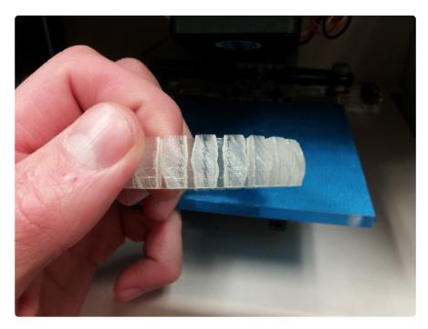
When the print job is complete, let your model cool or you might unintentionally mush it while prying it off the platform. If you model is stuck, use a plastic putty knife to carefully work around the perimeter of the object until it pops off. Clean up any excess material and you are good to go!
