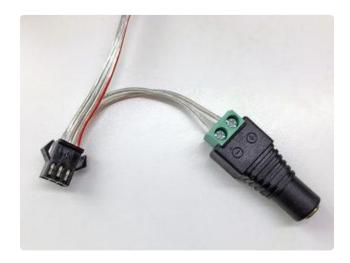
Connect a female DC power adapter using the screw connectors, being super extra careful to follow the polarity markings stamped on the DC jack:
