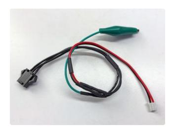
To connect the microcontroller at the "input" end of the strand, I soldered up this little adapter cable using a 3-pin JST plug (to the LEDs), a 2-pin JST cable (to the Circuit Playground, Flora or Gemma board) and one end of an alligator jumper cable.
