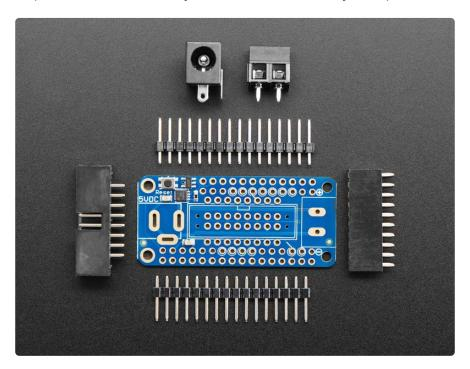
Each order comes with one FeatherWing PCB with surface mount parts attached, a 2x8 IDC header, a 2x10 female socket, 2.1mm DC jack, 5.08mm terminal block, and some male header. You may also want some <a href="Feather stacking headers">Feather stacking headers</a> () or <a href="female">female</a> headers () depending on how you plan to attach/stack your Feather.
