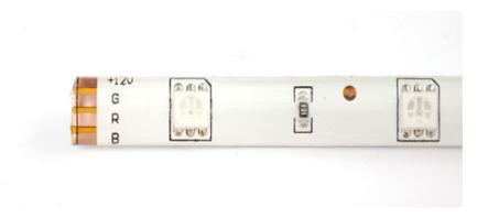
Cut away the waterproof overmolding at one end of the strip. The strips are symmetric so it doesn't matter which end you use.
