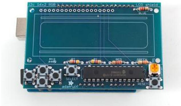
Solder all of the header pins. Even though they aren't used for passing signals, they will make the mechanical connection to the Arduino strong.
