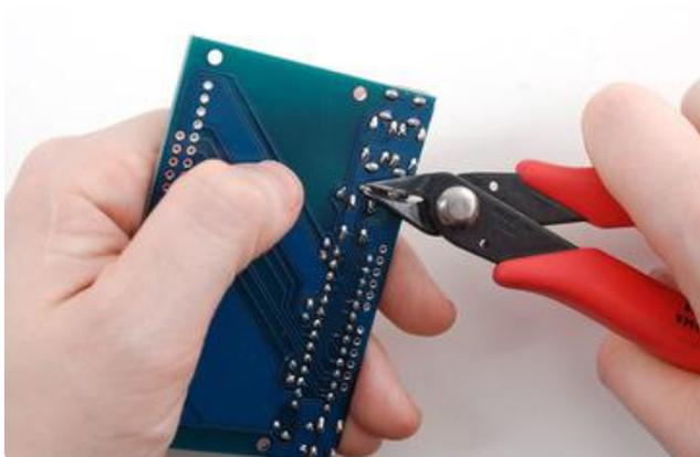
To make it sit flat, you may need to clip the legs of the buttons down - they will interfere with the DC jack, lifting the shield a bit.
