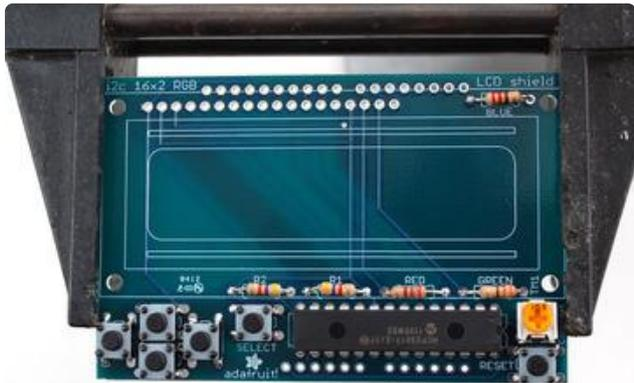
Unlike buttons or resistors, chips do have a direction and they must be put in the right way! First, use a flat table to carefully bend the legs of the chip so they are parallel. Then slip it into the silkscreened outline so that the notch at the end of the chip is on the right. Click the image to the left to make absolutely sure you've got it in the right way. Once you are sure, press the chip into place.
