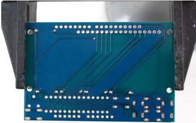
Flip over the PCB and check that all the legs for the buttons are sticking out.
