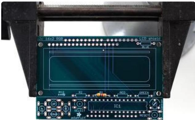
We'll start with the first resistor R1 - which has yellow, violet, red, gold bands on it. This resistor is part of the interface between the Arduino and the 'port expander' that controls the LCD.
