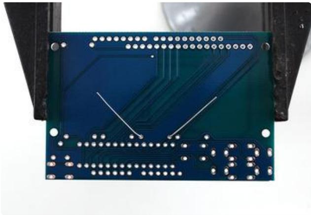
Bend the 'legs' of the resistor out so it sits flat against the PCB and flip it over.
