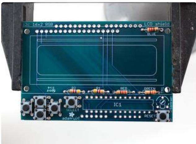
The button all the way to the right is the RESET button, for when you want to reset the entire system.
