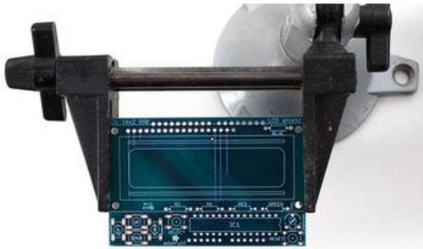
Put the printed circuit board into a vise or board holder, heat up your soldering iron and make sure you're ready to go!
