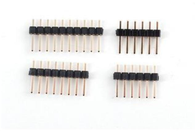
Take a stick of 36 pin header and break off a 10 pin piece, an 8 pin piece and two 6 pin pieces.
