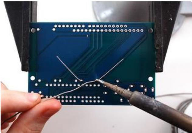
Then remove the solder and the soldering iron.
