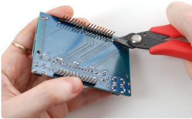
Finish up by carefully clipping the leads. For some Arduinos, the long leads may interfere with headers or parts on the Arduino board so we suggest just clipping them all. Do it carefully as these are a little difficult to cut and may fly at you. We suggest doing it over a trash can.
