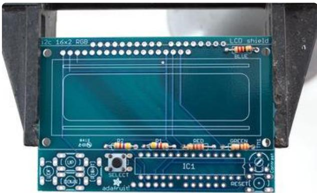
Next up we will place the buttons. These buttons are useful to send a signal to the Arduino (say if you have a basic menu system). We have a 4-way 'direction pad' for up/down/left/right input and a button to the right called SELECT. These 5 buttons should be able to make 'talking' back to your project easy. These are connected to the I2C port expander chip so they require no extra pins on the Arduino, our library does the work of reading whether they are pressed.
