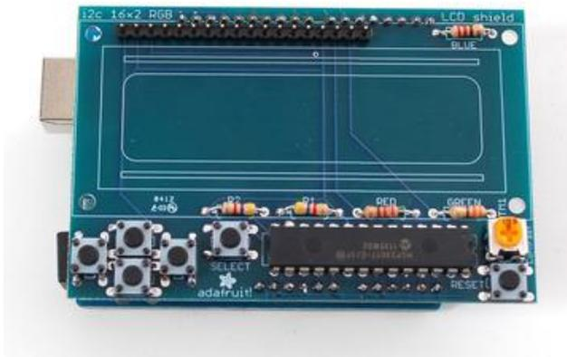
If you have an RGB 18 pin display break off a 18-pin strip of header and place it with the long ends down into the LCD placement slot.
