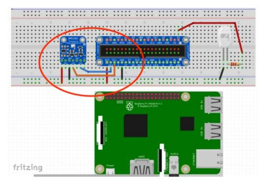
On the Pi Cobbler SDA is data pin and SCL is clock pin. On the BME280 sensor SDI is the data pin and SCK is the clock pin.
