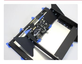
Set the "bow tie" carefully near the top of the screen. Pick up the driver board and... being very mindful of the flex cable, don't tear or pull it out...lower it on to the four small screws on the bow tie. Then add a nut for each.
