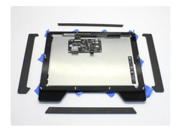
Another layer of edge pieces now fit over the screws and hold the screen from the back. These parts are symmetrical left to right and can go either way, but the top and bottom are unique. The wider edge should go at the bottom, and the right and left pieces should be flipped as needed to match.
