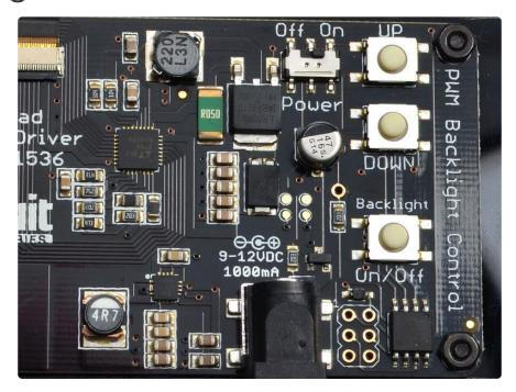
To control the backlight of the display, we use the awesome LT3754 LED driver from Linear Tech (https://adafru.it/d8V). The great thing about this driver is it is a cross between an efficient boost convert and a fully-matched constant-current LED driver. The boost converter half can take 9-12VDC and boost it up to ~22VDC and the LED driver half makes sure that each LED strand is driven with exactly 18.5mA for perfectly distributed light (which gives better color representation).
