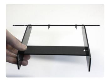
To reiterate a prior point: these screws should sit flush, pointing **back**, not forward. Getting this wrong will break the LCD!
