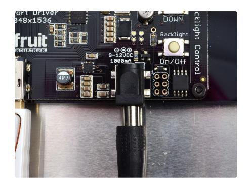
Once plugged in, check that the **POWER** switch is switched to **ON**. The power switch is in the upper right of this photo, next to the UP button
