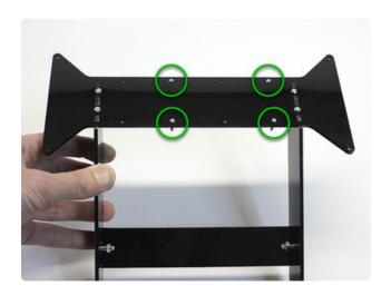
The "bow tie" has eight holes in it, but we'll only be using **four**. Looking at the flat side (the legs should poke out the back, not forward), install the four tiny #2-56 screws in the positions indicated here.
