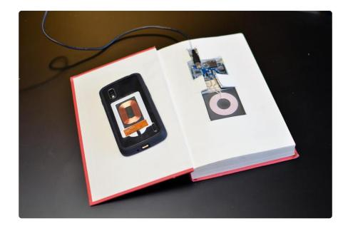
We'll put the charging module in the phone case and the charging transmitter inside the cover of the book. This project does involve some paper cutting with sharp blades, but is very simple. Let's get started!
