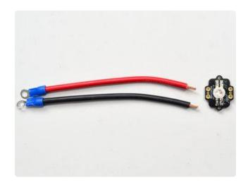
For the power wires, make sure to get nice hefty ones that can handle the current draw. Of course, it matters how long they're going to be, and how many Pixies are in the chain, and how much they will be lit up. 16 AWG is the recommended size.
