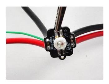
You can use a thinner wire for data, in this case we have a  $^{\sim}22AWG$  data line. It's soldered onto the out pin here
