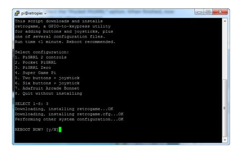
After rebooting, the HDMI monitor may display a "no signal" message. This is normal. Not all monitors can handle the resolution setting we're using. Once the PiTFT is wired up, that will be the primary display.
