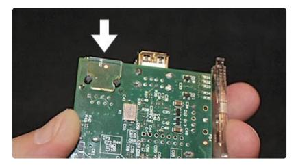
7. Position the bottom piece over the board, slotting it into the first side. There are no markings on the top or bottom piece — they are interchangeable and work in either orientation.
