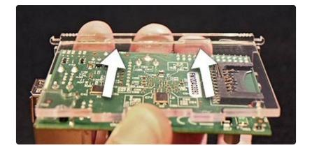
8. Turn the board over and install the top piece in a similar fashion. Or you can optionally leave the top off for full access to the GPIO and JTAG headers and the ribbon cable connectors.
