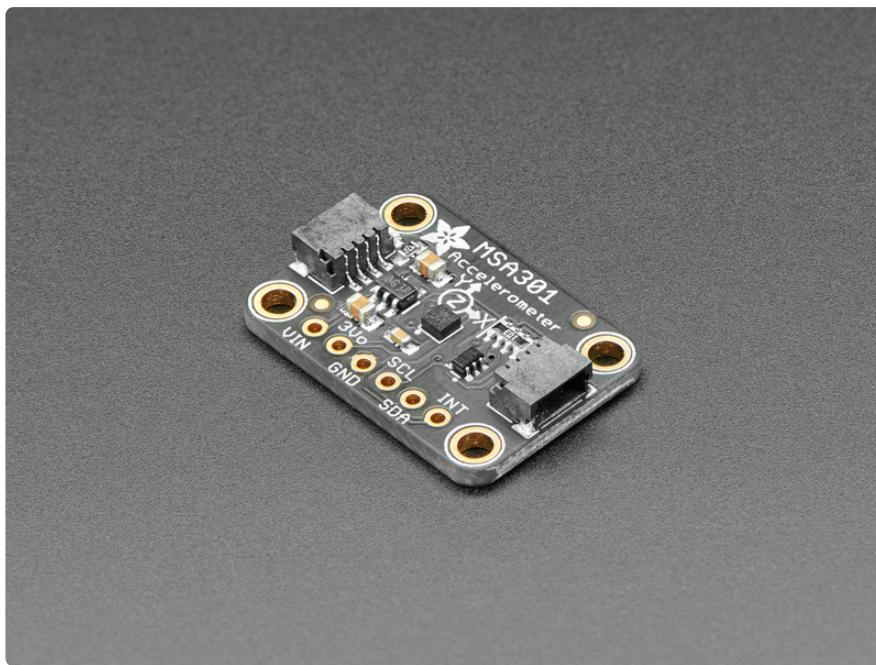
The MSA301 is a super small and low cost **triple-axis accelerometer**. It's inexpensive, but has just about every 'extra' you'd want in an accelerometer:
