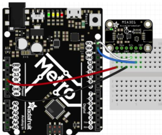
Connect **Metro or Arduino 5V** to board **VIN**
