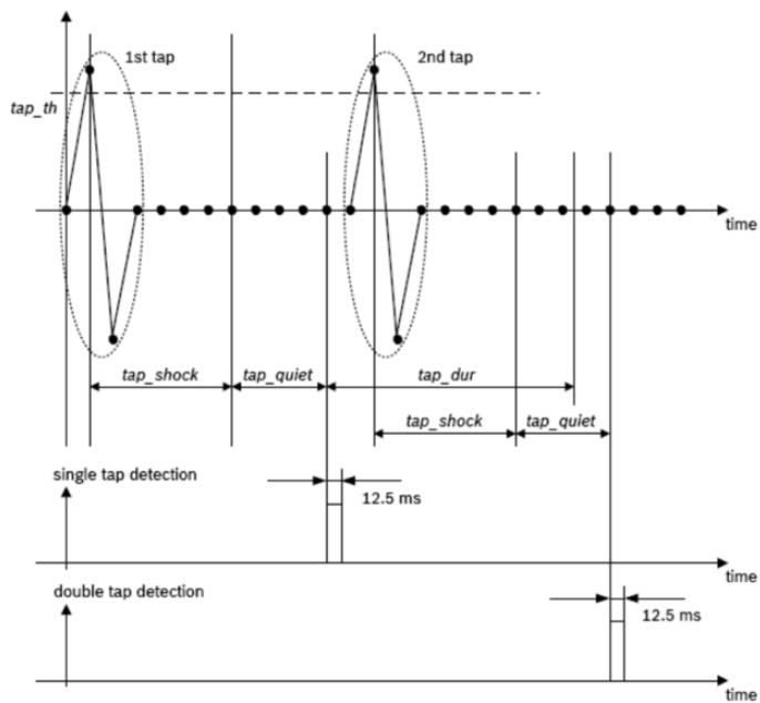
The tap detection parameters are set by calling **setClick**:
