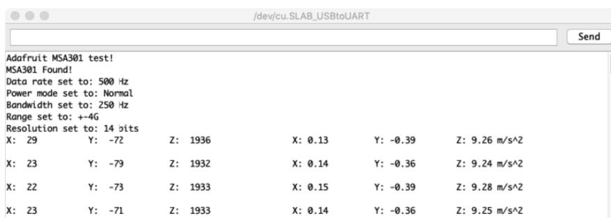
You can tilt the sensor in different directions to see the values for the different axes change.
