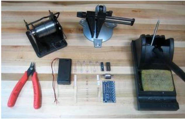
Get your space set up with a good light, a vice or "third-hand" tool, diagonal cutters, and a soldering iron/solder.
