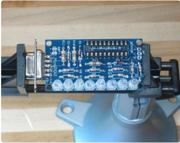
Next, place the microcontroller socket. Note that there is a little notch at the top, this tells you which way to put in the microcontroller. There is also a notch in the silkscreen image so match the two sides up, it will make it less likely for you to put the microcontroller in backwards (which could damage it).
