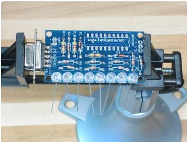
For the next step, you will place the 8 LEDs. LEDs have a 'direction' so if they're backwards they don't work. There are three ways to tell the direction.
