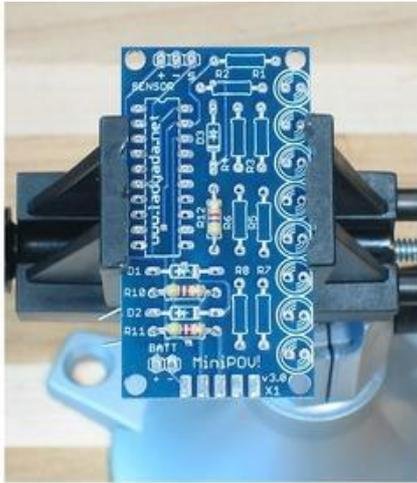
Place the 3 4.7K resistors as shown. Resistors are not 'directional' so don't worry which way they go in: it doesn't matter.
