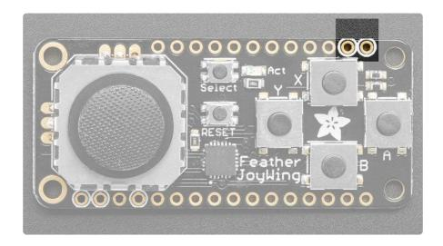
All data and control is done over I2C so it works with any and all Feathers! SDA and SCL are highlighted above. There are 10K pullups to 3.3V on each.
