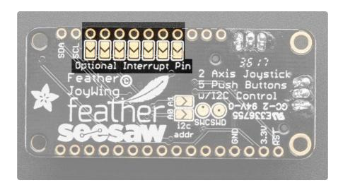
Soldering one of the jumpers for the optional interrupt will connect that pin of your Feather to the interrupt line on the Joy Featherwing. This will allow your Feather to know whether a button has been pressed or released without having to read each button over and over in a loop.
