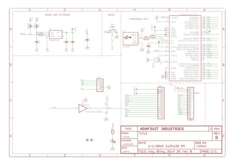
The 3.3V schematic regulator should be AP2112K-3.3
