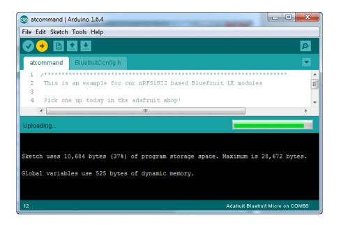
Don't click the reset button before uploading, unlike other bootloaders you want this one to run at the time Arduino is trying to upload
