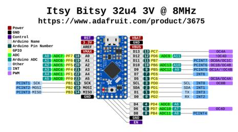
Click here to view a PDF version of the pinout diagram ()
