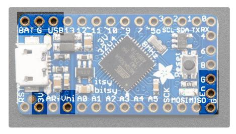
In addition to the three standard power pins, the 3V ItsyBitsy has a few more pins available for power sourcing:
