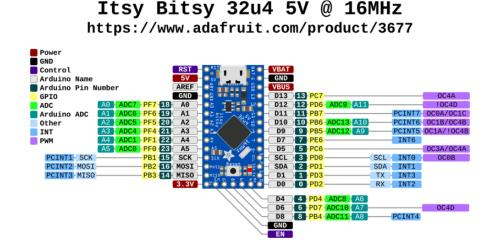
Click here to view a PDF version of the pinout diagram ()
