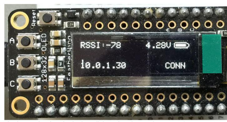
The data rendered on the display will depend on the way that you configure the example sketch, but the top and bottom lines are reserved for WiFi and LIPO information, and the two middle lines (referred to as the 'Message Area' in Adafruit\_FeatherOLED) can be used to render any text or messages.
