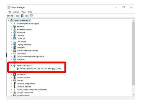
This check does not require any of the other software components we install later. So if a COM port is not showing up at this point, do not proceed further until determining why.
