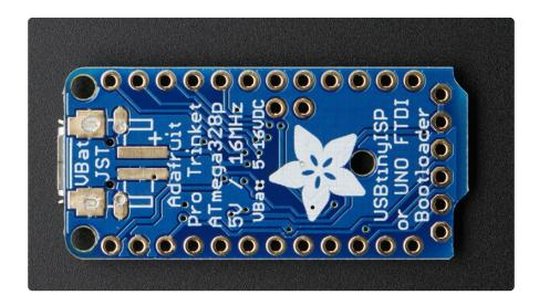
On the bottom there's a spot for a 2-pin JST-PH connector (http://adafru.it/1769). this is optional and can be soldered on by hand. It will let you use a lipoly or AAA battery pack (http://adafru.it/727) or a JST cable (http://adafru.it/261) for other power input. It's connected to the GND and VBAT pins
