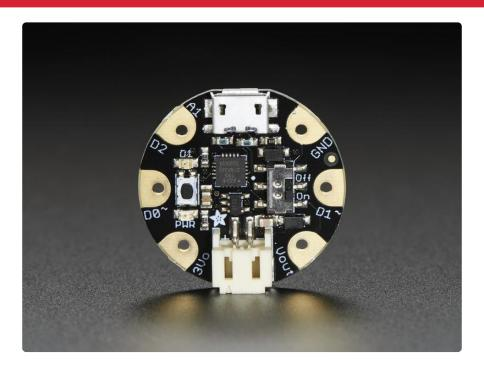
Don't forget to plug in the Gemma via a known-good USB cable to start the process. You should see the green power LED lit and the red bootloading LED pulse indicating that the Gemma is ready to start programming. If you've programmed the Gemma since getting it, you can always get it back to the bootloader state by pressing the small onboard reset button.
