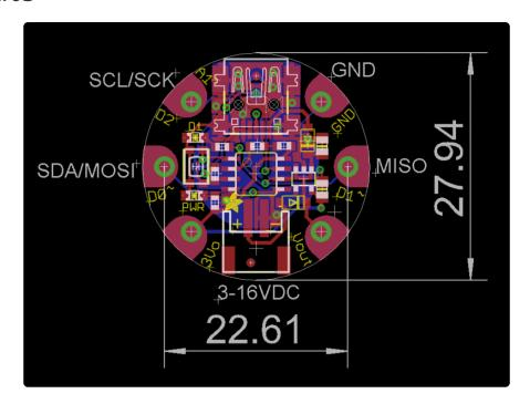
This diagram shows the physical size of the Gemma (diameter in mm) and the distance from pad to pad. The pads are at exact 90 & 45 degree angles except for 0 and 180 which is where the USB/JST connectors go
