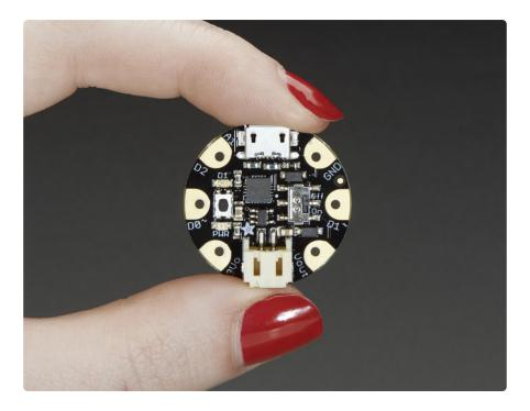
Love Flora but want a bite-sized version? Look no further, Gemma is a tiny wearable platform board with a lot of might in a 1" diameter package. Powered by a Attiny85 and programmable with an Arduino IDE over USB, you'll be able to realize any wearables project!
