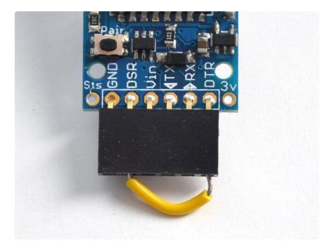
Then click on the DTR checkbox, this will toggle the DTR line on the EZ-Link, which will then feed back to the DSR line which will toggle the green DSR labeled box to the left. Make sure you see the green box turn on and off when you click the checkbox!
