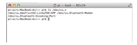
If you're using the Arduino IDE, it will show up under that name, use the cu. version not the tty. version
