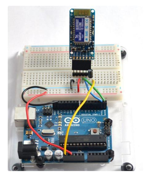
If you're using an Arduino compatible such as a Mini or Boarduino (or any of the other hundreds of Arduino-compat's), chances are it has an FTDI connector on it. You can plug the EZ-Link directly in, the GND pin lines up with the Black wire, and the DTR pin lines up with the Green wire. No other components are required
