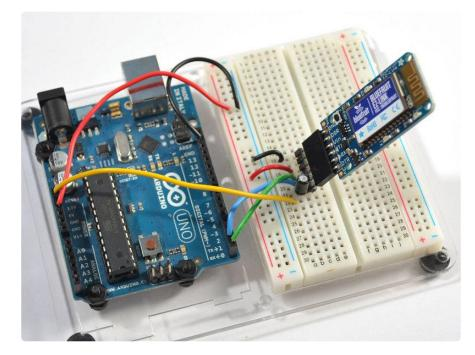
Unlike any other Bluetooth module, you can use the EZ-Link to program an Arduino. The reason this is possible is because EZ-Link can dynamically change the baud rate and has the ability to send the DTR signal from the Arduino IDE wirelessly through the module. Both are required if you want to be able to quickly change to the 115.2K signal required for upload and toggle the DTR lines.
