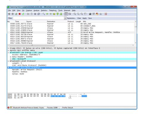
What this write request is trying to do is enable the 'notify' bit on the <u>UART service's TX characteristic</u> (https://adafru.it/iCn) (0x001E is the handle for the CCCD or '<u>Client Characteristic Configuration Descriptor</u> (https://adafru.it/ecl)'). This bit enables an 'interrupt' of sorts to tell the BLEFriend that we want to be alerted every time there is new data available on the characteristic that transmits data from the BLEFriend to the phone or tablet.
