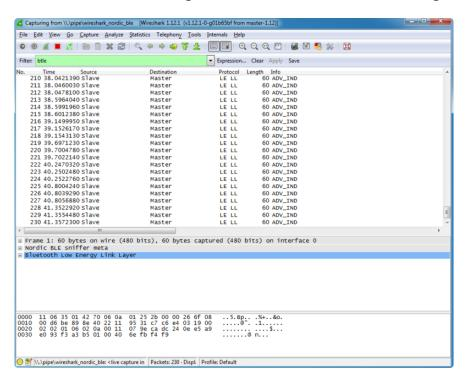
One of the key benefits of WireShark as an analysis tool is that it understands the raw packet formats and provides human-readable displays of the raw packet data.
