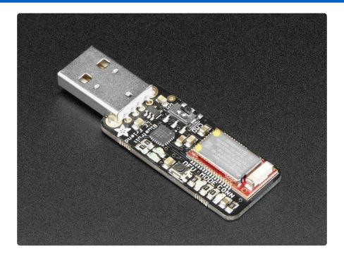
In it's simplest form, it works on the same principle as a common USB/Serial adapter (the <u>FTDI Friend</u> (https://adafru.it/dQa), for example!). Any data that you enter via your favorite terminal emulator on your development machine will be transferred over the air to the connected phone or tablet, and vice versa.
