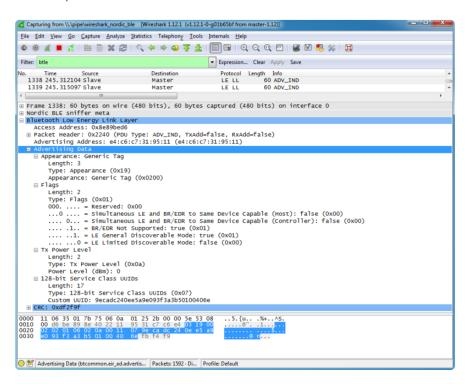
Clicking on the Advertising Data entry in the treeview will highlight the relevant section of the raw payload at the bottom of the screen, but also provides human readable information about the payload that can save you a lot of time trying to debug or reverse engineer a device.
