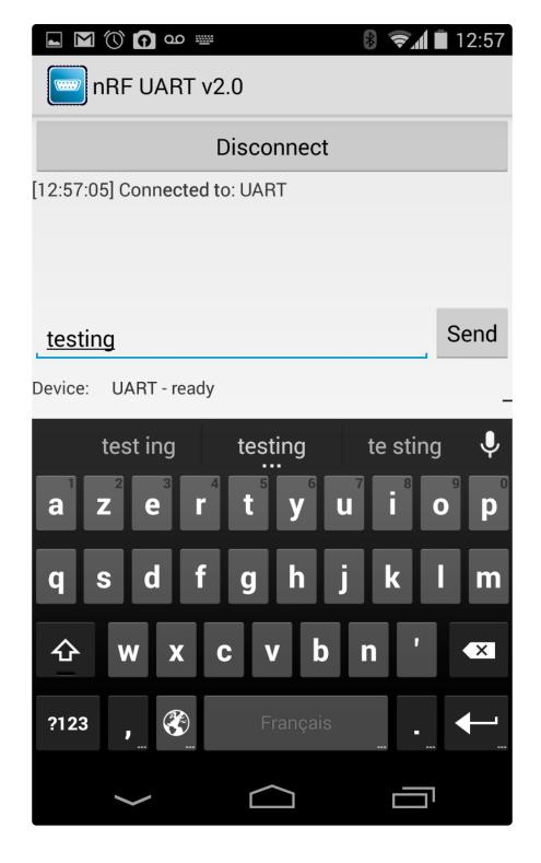
On the BLEFriend side we can see the 'testing' string that was sent from nRF UART in the terminal emulator below:
