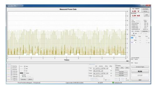
The MODE LEDs can be seen blinking in regular intervals as the three rectangular bumps at the bottom of the chart.
