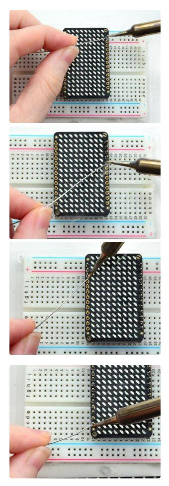
Solder in the two long header strips. Not all are connected on the LED matrix but it makes the connections mechanically stable.
