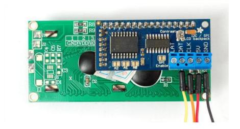
For advanced users, this project can be used for general purpose I/O expansion, the MCP23008 has 8 i/o pins (7 are connected) with optional pullups, the SPI 74HC595 has 7 outputs.
