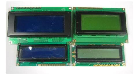
This backpack will work with any 'standard'/'classic' character LCD. It does not work with graphic LCDs. Character LCDs come in sizes ranging from 8x1 (8 characters, one line) to 40x4 (40 characters, four lines). The backpack will also only fit LCDs that have a single line of pins at the top, not the ones that have a 2x10 or 2x8 connector on the side. Those are much rarer these days but just keep a look out for that!
