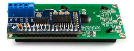
Make sure that as you solder the first pin, the backpack PCB isn't leaning against the LCD, where the terminal blocks could short against some components. You can put some electrical tape or foam tape behind to avoid this if you think it could be an issue.
