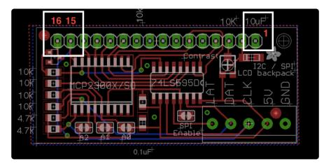
If your LCD has 18 pins, you won't be able to use the extra backlight pins, just connect 1-16 and leave 17 and 18 disconnected
