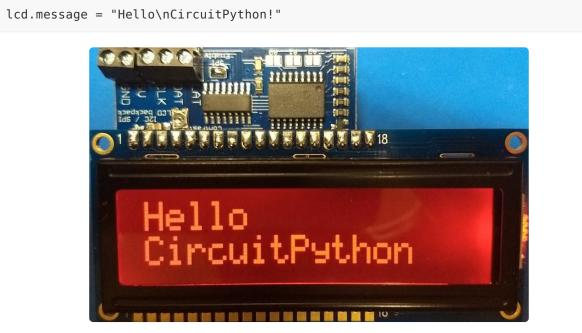
See the parallel LCD guide for more functions you can call to control the LCD! (https://adafru.it/CVQ)
