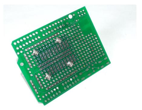
Solder wires from each pogo pin to a matching pin on the shield. For this SD card interface I connected the SPI pins to the SPI port. Then the output of the 3.3v regulator goes to an analog pin. I also connected the card detect pin up so I can tell when a board is being tested.
