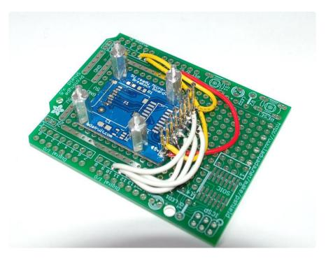
A piezo buzzer is connected to pin #9 (underneath the PCB).
