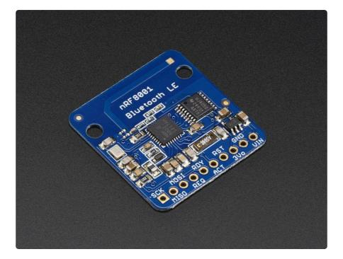
Our nRF8001 Breakout allows you to establish an easy to use wireless link between your Arduino and any compatible iOS or Android (4.3+) device. It works by simulating a UART device beneath the surface, sending ASCII data back and forth between the devices, letting you decide what data to send and what to do with it on either end of the connection.
