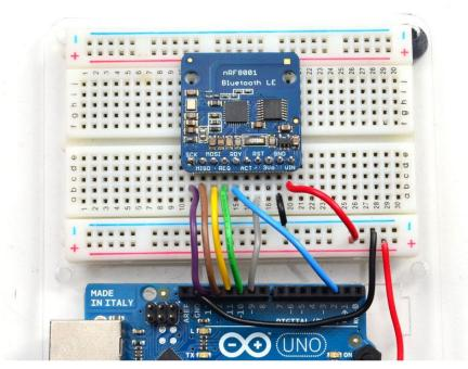
The nRF8001 differs from a classic SPI bus since CS is replaced by two pins, REQ and RDY, but you can still use HW SPI since CS is normally controlled purely in SW anyway.
