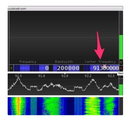
This will bring a range of frequencies into view -- approximately 3MHz at a time are available. Now, you can set a demodulator down on a range you want to tune. This is done by clicking in the waterfall display, with the cursor at the center of the frequencies you want to hear. This will usually be the orange and red display section, showing you where the strongest signal lies.
