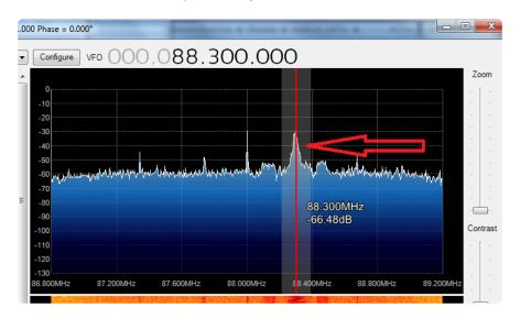
With the latest versions of SDR-Sharp it will automatically detect and decode RBDS/RDS data that is sent along with FM radio
