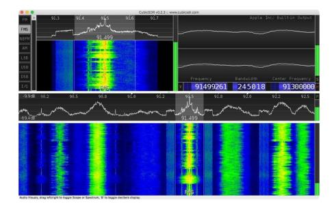
You can see the fine tuning section in the upper left corner gives us a zoomed in view of the demodulator. You can drag this one left and right in the waterfall section to fine tune, or grab one of the outer edges of the demodulator to change the bandwidth that is being processed. Too wide and you'll pick up unwanted signals, too narrow and you'll start to cut off important parts of the signal.
