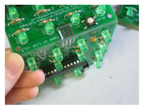
Bend the wire down and solder it to the second board.
