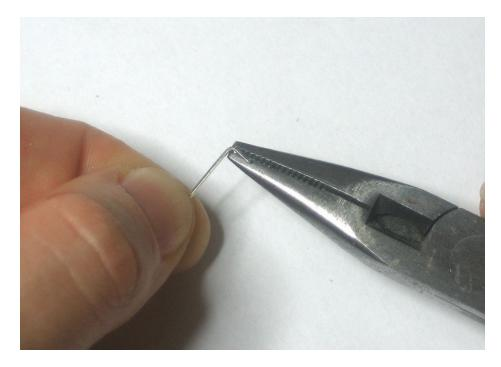
Thread it through the adjacent holes, then solder to make a connection to both boards.
