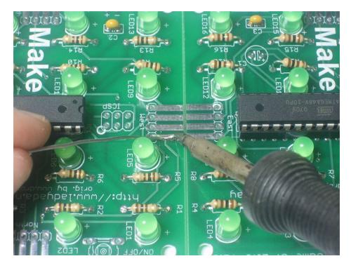
Then drag the soldering iron between the two boards, and slowly lift it in the middle.
