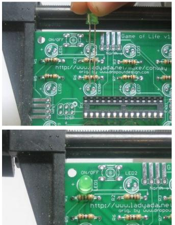
Next are the LEDs. LEDs, unlike resistors, are polarized and must be placed correctly or they won't light up. One leg of the LED is slightly longer than the other. This is the positive (+) leg. If you look at the image on the PCB, you'll note that one side has a + next to it, this tells you how to orient the LED. Make sure the long lead goes in the hole marked +.
