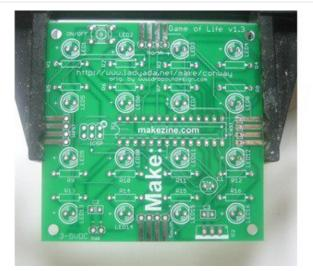
Take the PCB and place it in a vise or other holder so that you can easily place and solder parts.
