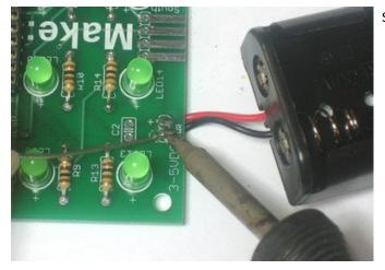
Solder in the two wires.
