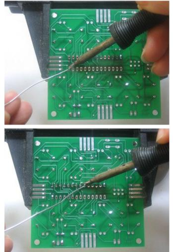
The socket has short legs so it's more likely to slip than a resistor. The easiest way to solder the socket is to hold it against the PCB with one finger (or tape) then solder in two points on opposite sides. Once you've got it tacked, solder in the remaining pins.
