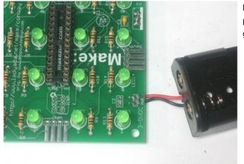
Next, connect up the battery pack. The red wire of the pack goes to the hole marked with a +, the black wire goes to ground, marked with a -.
