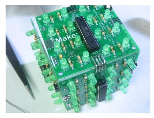
Test the cube after each new board to make sure you've got it on right.
