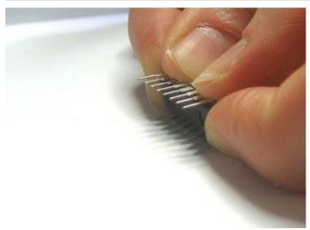
Next it's time to insert the microcontroller that does all the hard work of calculating the game and displaying LEDs. Chips come from the factory with their legs angled out, so press against a flat table top so that the legs are straight and parallel.
