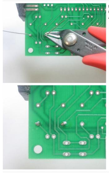
Put down the iron and pick up the diagonal cutters. Using the cutters, clip the wires of the resistor right above the joint.
