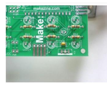
Next we're going to place the ceramic capacitor **C3** and the wire jumper for **IC2**.
