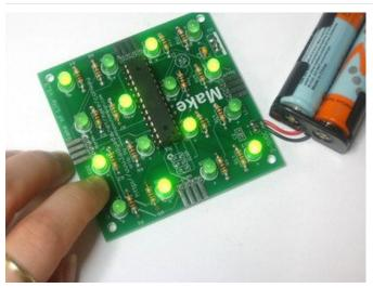
Time to test! Place two AA batteries (rechargables or alkalines) into the pack and watch the Game of Life start playing. If you press the ON/OFF button you should see a checkerboard pattern.
