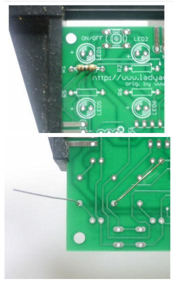
The resistors are named R1 thru R16. Placing them on the PCB is easy, just look for the image on the PCB that matches the shape of the resistor. Resistors are **nonpolarized** that means you can stick them in 'either way' and they'll work just fine.
