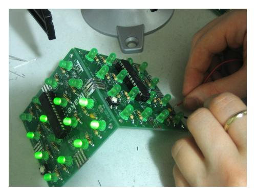
Connect a third board. The trick to knowing how to orient boards is that you can always connect **North** and **East** & **South** and **West** ports together. In this case we connect West and North of the new board to the existing structure.
