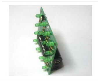
Stick the battery pack onto the back of the PCB, near the bottom. That way the weight of the batteries will act as a stand so that the kit can sit on your desk!
