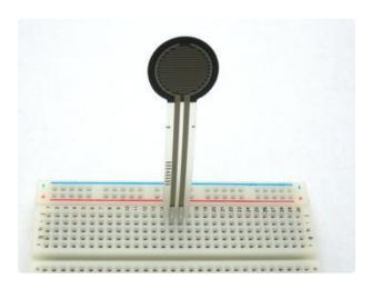
FSRs are often a polymer with conductive material silk-screened on. That means they're plastic and the connection tab is crimped on somewhat delicate material. The best way to connect to these is to simply plug them into a breadboard.
