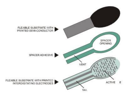
FSRs are basically a resistor that changes its resistive value (in ohms  $\Omega$ ) depending on how much it is pressed. These sensors are fairly low cost, and easy to use but they're rarely accurate. They also vary some from sensor to sensor perhaps 10%. So basically when you use FSRs you should only expect to get ranges of response. While FSRs can detect weight, they're a bad choice for detecting exactly how many pounds of weight are on them.
