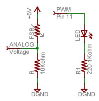
This sketch will take the analog voltage reading and use that to determine how bright the red LED is. The harder you press on the FSR, the brighter the LED will be!
