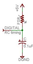
In this case, our 'bucket' is a 0.1µF ceramic capacitor. You can change the capacitor nearly any way you want but the timing values will also change. 0.1µF seems to be an OK place to start for these FSRs.
