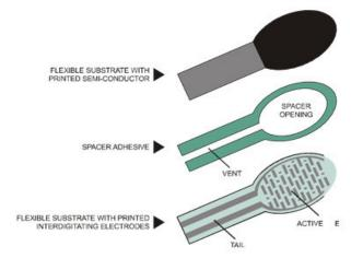
FSRs are basically a resistor that changes its resistive value (in ohms  $\Omega$ ) depending on how much it is pressed. These sensors are fairly low cost, and easy to use but they're rarely accurate. They also vary some from sensor to sensor perhaps 10%. So basically when you use FSRs you should only expect to get *ranges* of response. While FSRs can detect weight, they're a bad choice for detecting exactly how many pounds of weight are on them.
