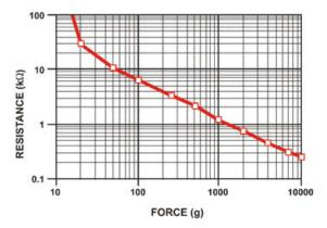
It is important to notice that the graph isn't really *linear* (its a log/log graph) and that at especially low force measurements it quickly goes from infinite to  $100 \text{K}\Omega$ .
