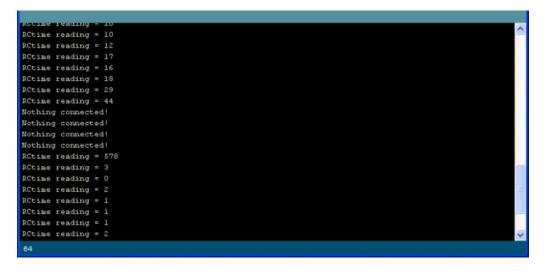
It is possible to calculate the actual resistance from the reading but unfortunately, variations in the IDE and arduino board will make it inconsistant. Be aware of that if you change IDE versions of OS's, or use a 3.3V arduino instead of 5V, or change from a 16mhz Arduino to a 8Mhz one (like a lilypad) there may be differences due to how long it takes to read the value of a pin. Usually that isn't a big deal but it can make your project hard to debug if you aren't expecting it!
