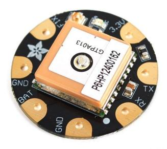
This module is the best way to add a GPS to your wearable project. It's part of the Adafruit Flora series of wearable electronics, designed specifically for use with the Flora motherboard. Installed on the PCB is the latest of our Ultimate GPS modules, a small, super-thin, low power GPS module with built in data-logging capability! This module's easy to use, but extremely powerful:
