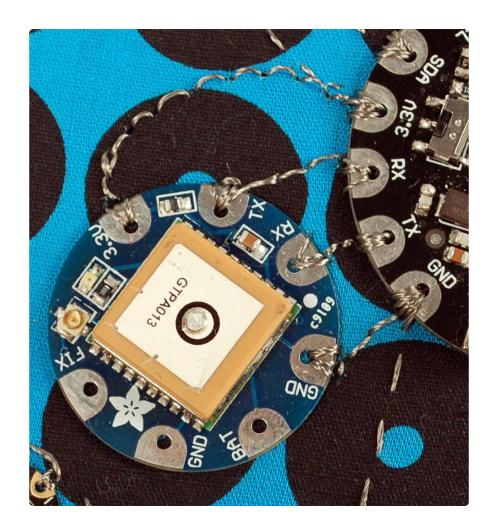
The four connectors are all in a row just to the left of Flora's JST battery connector for easy sewing. But test your project with alligator clips before sewing it in!
