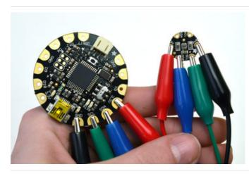
To test the sensor before sewing it into a project, use alligator clips to hook up the 3.3v, SDA, SCL, and GND pins.
