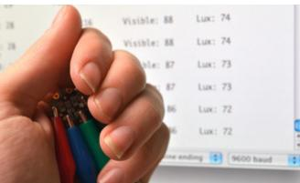
Open the serial monitor (the upper right button in the Arduino IDE) and watch the sensor values pour in.
