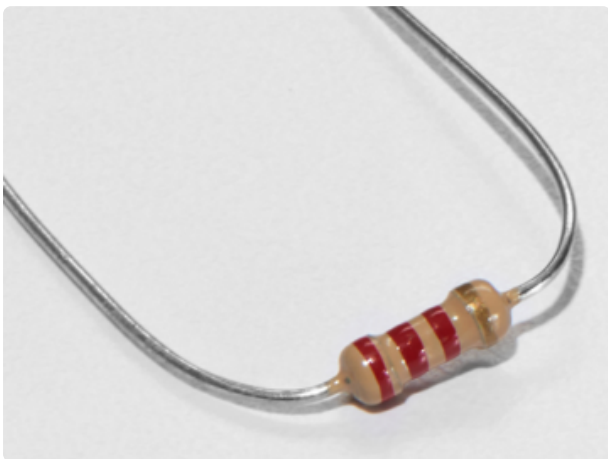
2.2k Ohm Resistor
