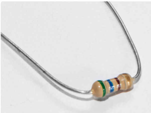
560 Ohm Resistor Colors: Green > Blue > Brown
