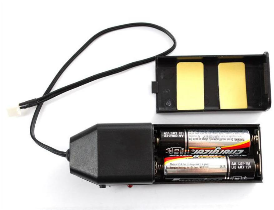
The voltage should be between 50-120V AC RMS (150V-360V peak-to-peak). Higher voltages result in a brighter display (but lower overall wire-life).
