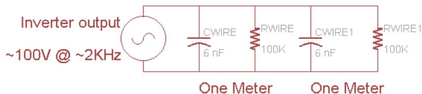
Of course, we can simplify by calculating the new capacitance and resistance. Remember that capacitance increases in parallel and resistance decreases.
