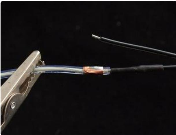
Now we can revisit the corona wires. Using the tip of the soldering iron, heat up the copper tape and melt a little solder on.
