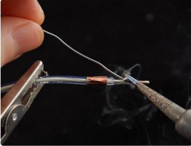
Now tin the wire by heating it up with the soldering iron tip and melting solder onto the wire, this will coat it with solder - makes it easier later to solder on the wire.
