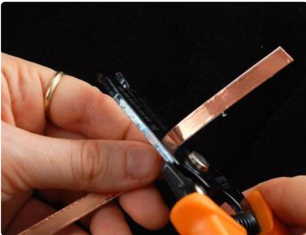
Next, cut a 1" or so piece of 1/4" copper tape. Dont use scissors to cut copper tape, use wire cutters!
