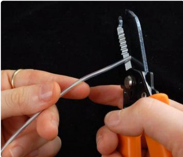
Start by cutting the wire to be as long as you want, and add an inch (or if you're starting out, a few inches) for the wire connection. Remember, its very easy to make the wire shorter but hard to make it longer!
