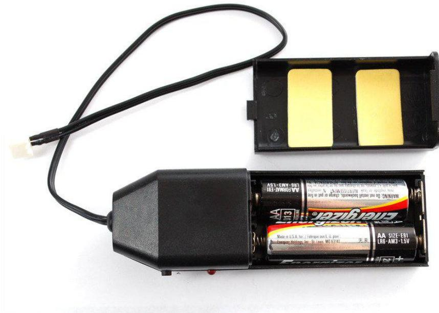
This pocket inverter can drive approximately 1 to 15 feet (0.3-5 meter) of 'classic' EL wire such as LyTec. Since we are using higher-brightness EL wire in the shop, it can only drive half as much, 1 to 7.5 feet (0.3 to 2.5 meter). We found that 2 meters gives a nice bright glow at good voltage and frequency. At 3 meters, its not as bright, it appears about the same as 'classic' EL.
