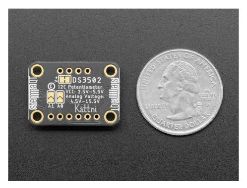
"OK, this thing sounds great. Give me some details" you say. OK then, here you go: The wiper value is a 7-bit number meaning there are 128 possible levels of resistance to choose, from 0-10K ohms. You can even set a default value that will be set on power up. The analog voltage controlled can be from 4.5-15.5V. Additionally you can use the address jumpers or pins to set the I2C address to one of four values, allowing you to have four DS3502s on the same I2C bus.
