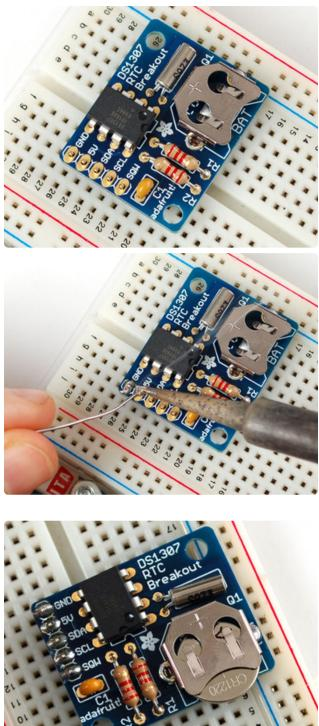
If you'd like to use the header to plug the breakout board into something, place the header in a breadboard, long side down and place the board so that the short pins stick thru the pads.
