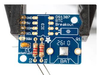
Place the two 2.2K resistors, and the ceramic capacitor. They are symmetric so no need to worry about direction. If you're planning on using with a Raspberry Pi (which has 3.3V logic and built in pull-ups, skip the 2.2K resistors!
