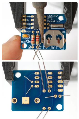
To keep the battery holder from falling out, you may want to 'tack' solder it from the top.
